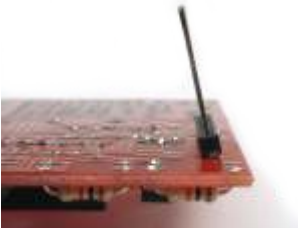
Pin strip installed crooked - good thing you soldered only one pin!
