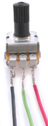
Usually this type of device has three connections. If you measured the resistance across the two outer terminals it would be constant. The resistance between the middle terminal and either of the outer terminals varies. In the image of the potentiometer, the red wire is the + 5 volts, the black wire is Ground, and the green wire is the analog signal.
