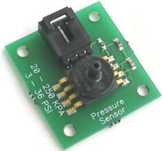
A wide range of analog sensors are offered, all designed to plug into the PhidgetInterfaceKit 8/8/8 board. The PhidgetInterfaceKit 8/8/8 board can be controlled from Windows, Linux, and Mac OS X. High-level programming interfaces are available for Visual Basic, C, C++, Flash, .NET, Java, LabVIEW, etc.
