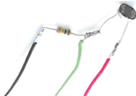
Here, our variable resistor is  $R_v$  and our constant resistor is  $R_c$ . Our measurement point 'A' is at the connection between the two resistors. Again let's start with the Ohm's Law:
