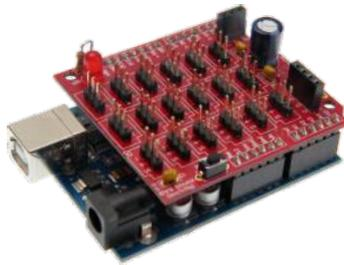
SB-GVS Shield on Arduino
