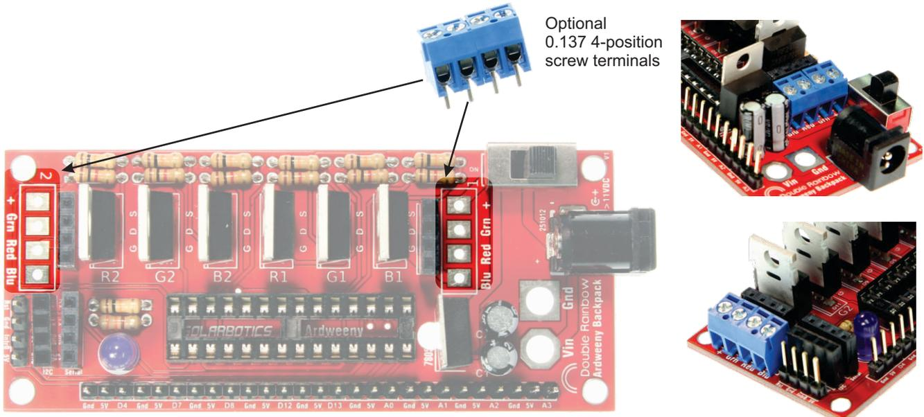
**Step 9 - Da Ardweeny!:** Plug the Ardweeny into the socket, with its LED closest to the PCB's blue LED. Add code. Add RGB Strips. Add power. BEHOLD THE DOUBLE RAINBOW!
