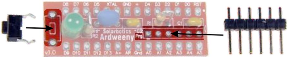
Step 6: Install the Reset Switch
