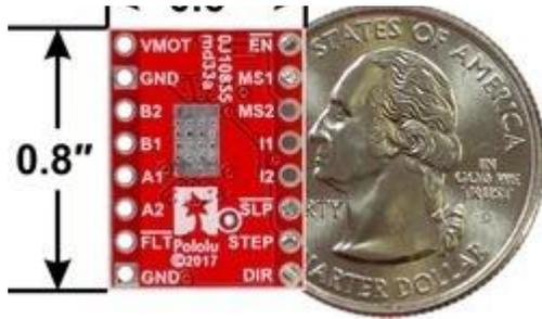
**MP6500 Stepper Motor Driver Carrier, bottom view.**
