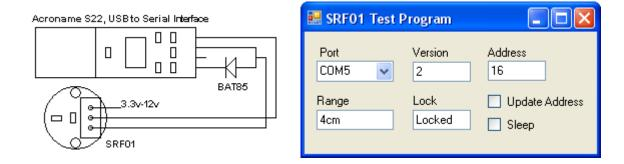
We have a small test program, written in C# which controls the SRF01 via an Acroname S22 module. A small schottky diode is used to prevent the SRF01 trying to drive the S22's output line (data from the PC). You will need to download and install the <u>FTDI VCP</u> drivers to use the S22.
