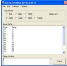
In this program the 'init' section sets the serial pin high and then waits for 100ms. This gives the XBee time to 'reset and wake up'. The main loop then reads the light value (readadc on input0) and temperature value (readtemp on input1) and transmits the data every second.
